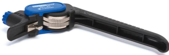
The Dismantling Tool No. 25 was developed for stripping cables with sheath thickness of up to 5 mm. The cutting blade can be used for round and length cuttings. For the round cut a minimum cable diameter of 25 mm is necessary.
