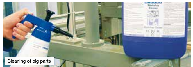
Cleaning of parts to be bonded
